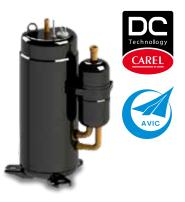
**Operating range** Evaporation temperature: -35T25 °C Condensing temperature: -13T82 °C
