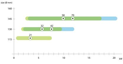
0/75 °C= evaporation temperature/condensing temperature 10/5 K= superheat/subcooling •= capacity values at 60 rps
